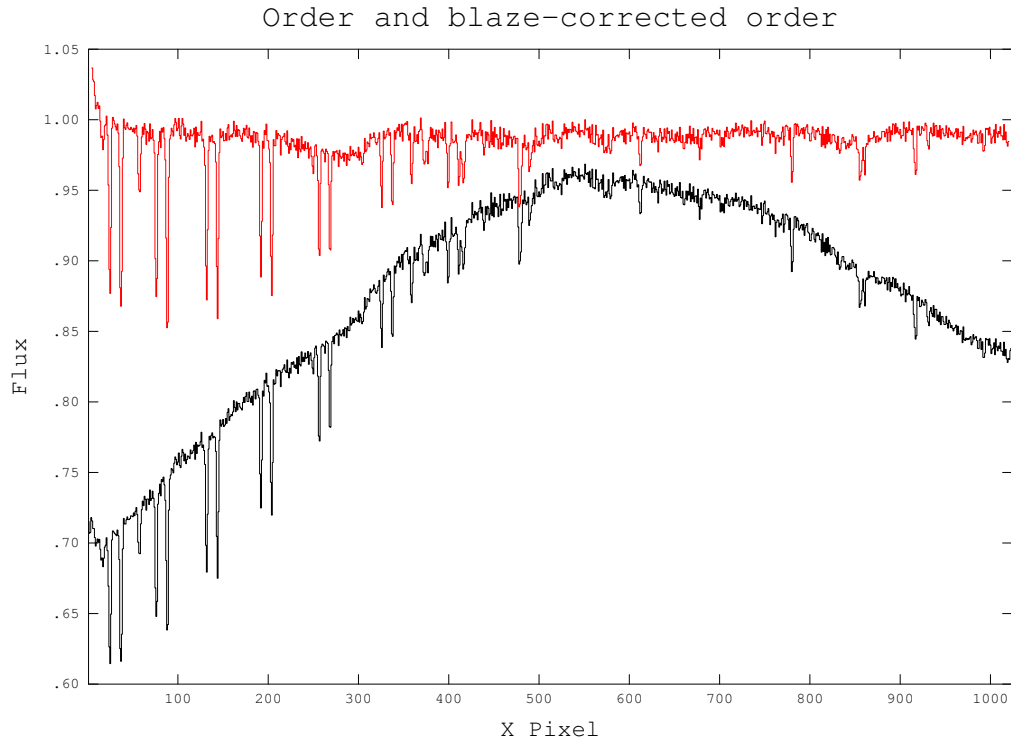
Figure 7: Blaze correction: the top spectrum is the blaze-corrected version of the lower spectrum. Note that the flux values in the uncorrected order have been scaled and shifted for this plot.
